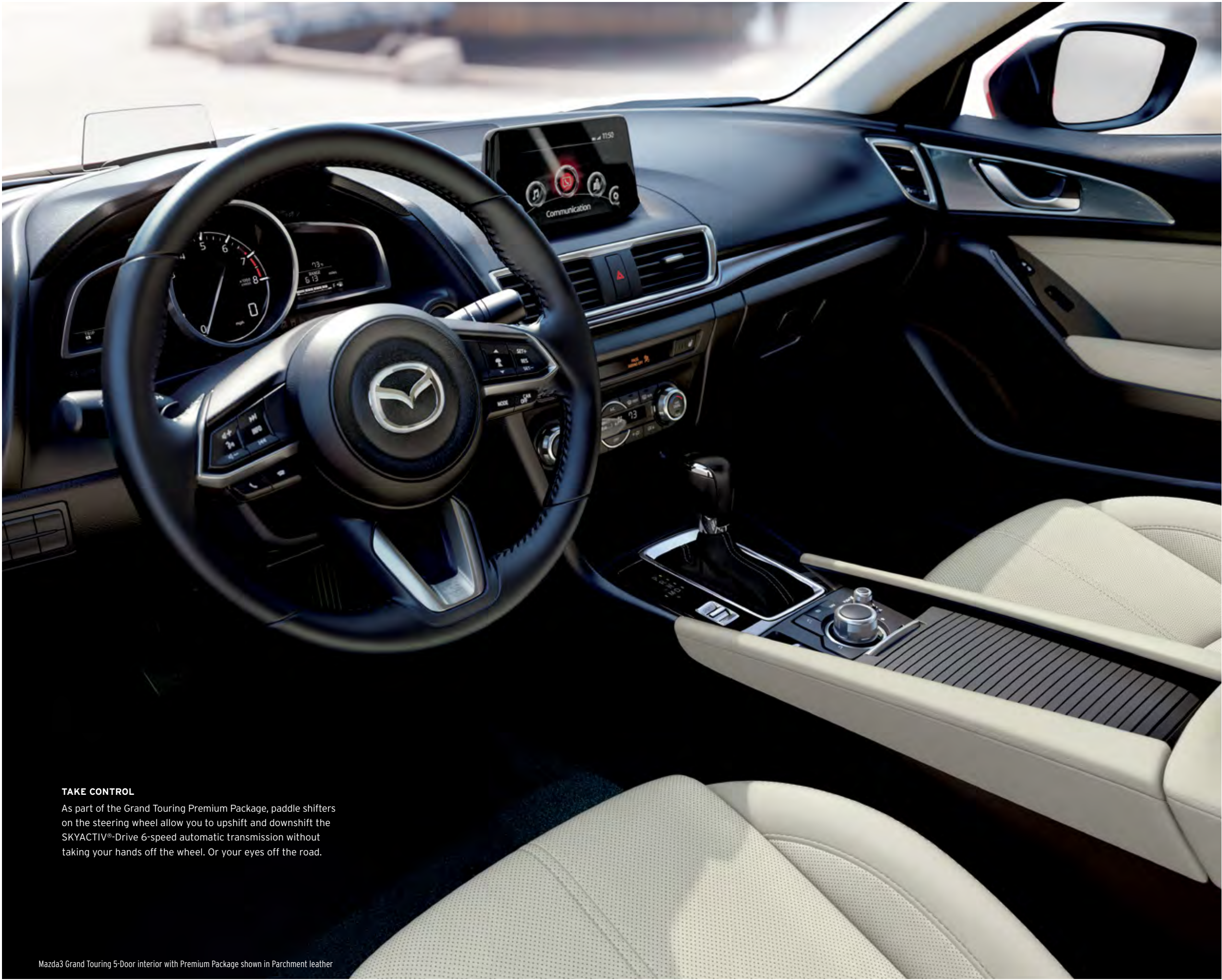
Information displayed: vehicle speed, tachometer, navigational directions, safety alerts, cruise control data and speed limit information (when available)
